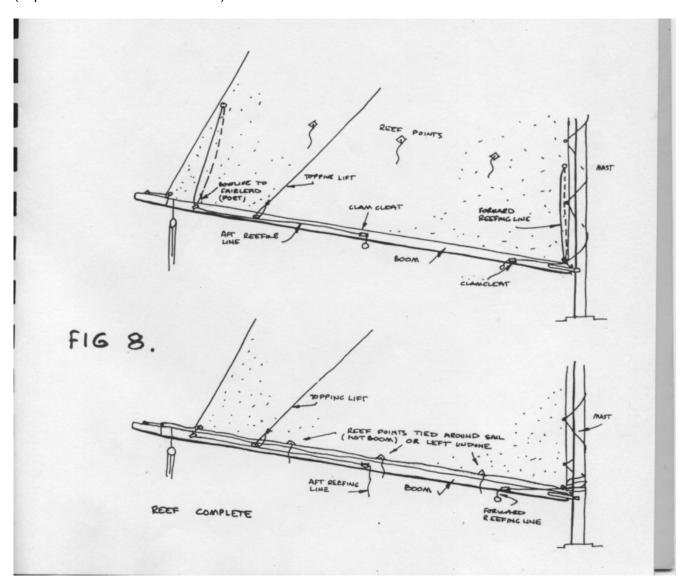
The Cormorant employs a slab reefing arrangement for her single reef and you will find a short and a long reefing line, each fitted with a coloured plastic parrel bead in the kit of loose items supplied with each boat.
